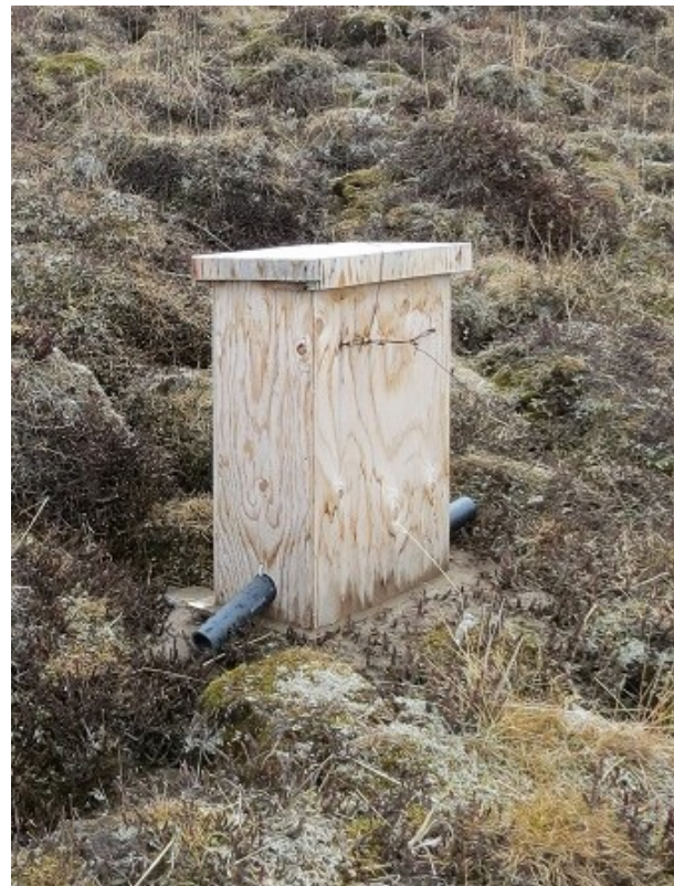
Wooden box holding an automated camera.
